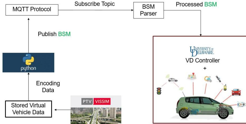
Figure 2.22: Bench test model emulating the virtual reality based field test.
