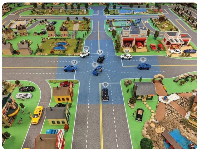
FIGURE 1 A view of the Information and Decision Science Lab Scaled Smart City, with connected and automated vehicles coordinating at an intersection.
